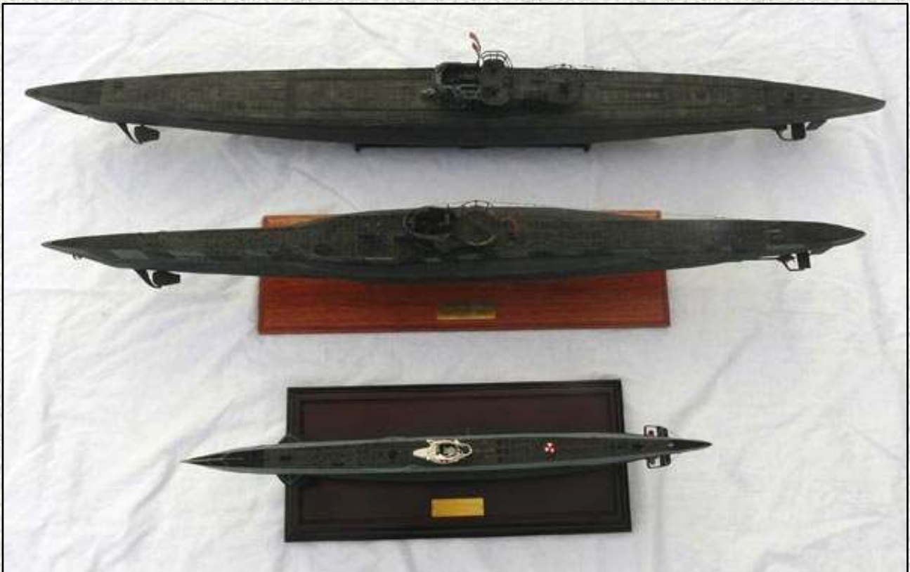
Above (1): A 1/72 nd scale Wolf Pack of the three main U-boat types: the large ocean-going Type IXC, medium ocean-going Type VIIC and small coastal Type IIA.
