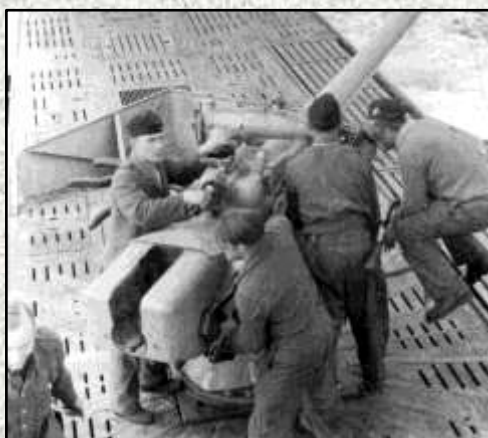
Above (B53): An unidentified Type IX with crewmen operating the 105mm deck gun. In this circumstance both the sides have been removed leaving only the central section in place.
