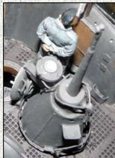
Right (E59): An eagle eye view of the attack periscope housing, clearly showing the wooden shelf in the extended position.
