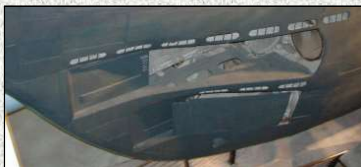
Above (B62): A somewhat damaged U 67 in October 1941. While some vents have been lost due to damage to the bow, this boat had port pattern A which was commonplace at the time. Above right (B63): The museum boat U 505, which presently has port pattern E, originally had port pattern B. Pattern E is unique, being formed due to years of corrosion in Chicago which resulted in one vent being covered over.
