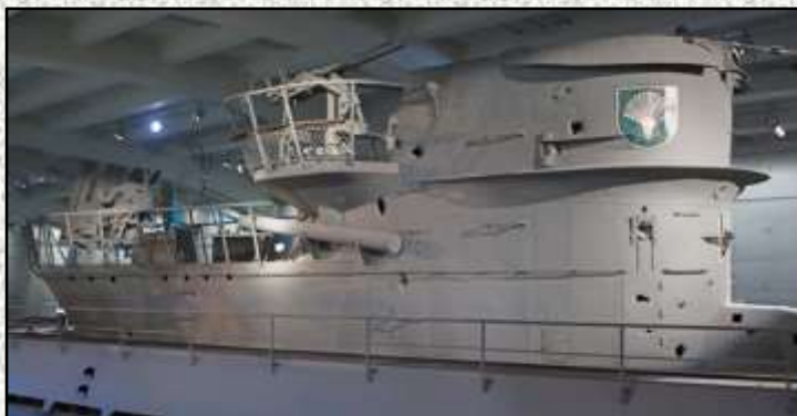
Right (B96): U 505 under cover in Chicago with a Turm IV tower which replaced the boat's Turm II.
