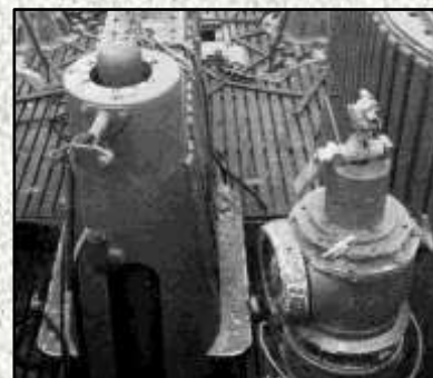
Above (B105): The newer style of UZO column was offset to port on Type IXs.
