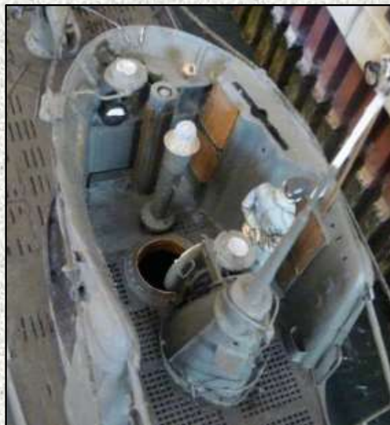
Above (E58): Many details can be discerned in this photo. The two magnetic compass repeaters - one directly in front of the attack periscope housing and the other near the front of the tower - can be seen. Below the front repeater is a cable to the boat below and a black and white dial. Over the right hand side of the "dashboard" area is a brass voicepipe on a scratchbuilt shelf.
