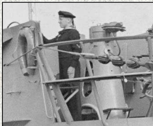
Above (B31): The commissioning of U 103 in July 1940. The semi-circular drainage gap at the bottom of the periscope housing can clearly be seen along with a substantial rim at the edges. The C-shaped ring and two support bars below can be seen at the bottom of the rear end of the periscope housing.
