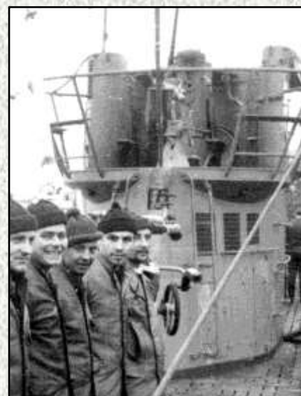
Above (B28): This later shot of U 108 shows that the metal seats have been replaced by a ledge low down on the bulwarks and on each side of the periscope housing.
