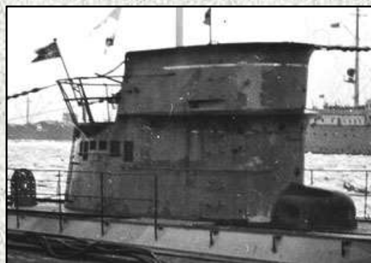
Above (B2): A full length spray deflector is in place on this wartime IXA but the top of the tower still does not yet have a wind deflector.
