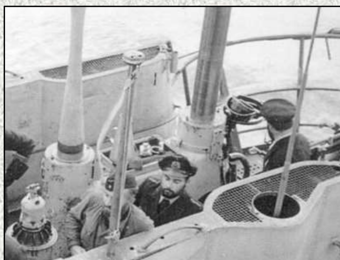
Above (B7): Style Z1 on U 129 in April 1942 clearly shows the criss-cross mesh grill and the periscope rod aerial in the raised position.
