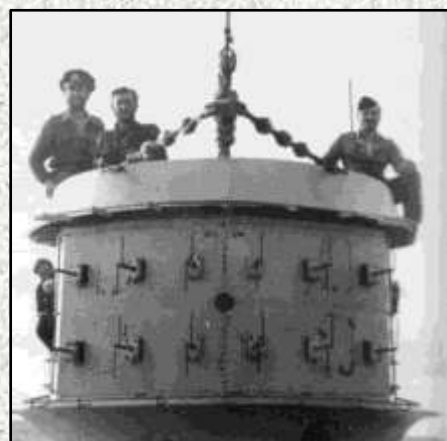
Above (B88): A frontal view showing the FuMO 29 dipoles and baseplate on an unidentified IXC.
