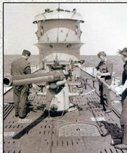
Above (B42): The access hatch is clearly offset to port ahead of the 105mm deck gun.
