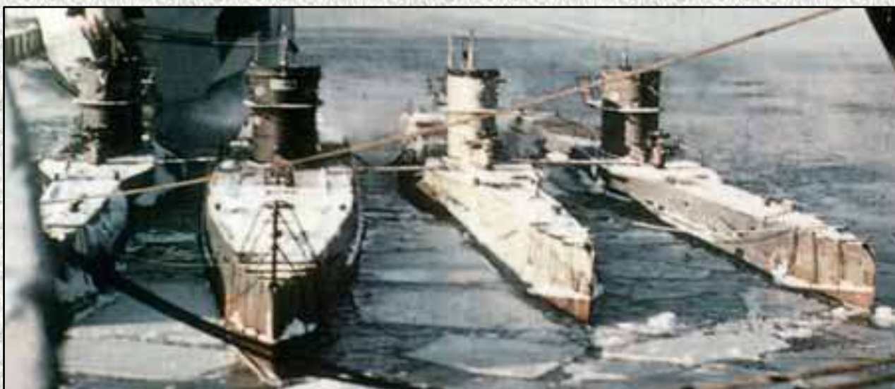
Above (A7): The U-boats seen here in Gotenhafen have rusty protective caps over their bows to prevent damage from ice. The decks are covered under a layer of snow. The Type IX second from the left, U 37, looks particularly dark.
