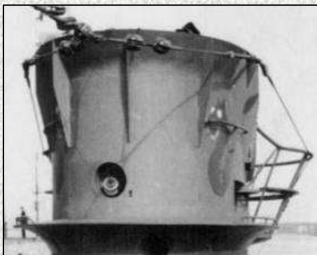
Left (C16): An experimental wind deflector on U 71.
