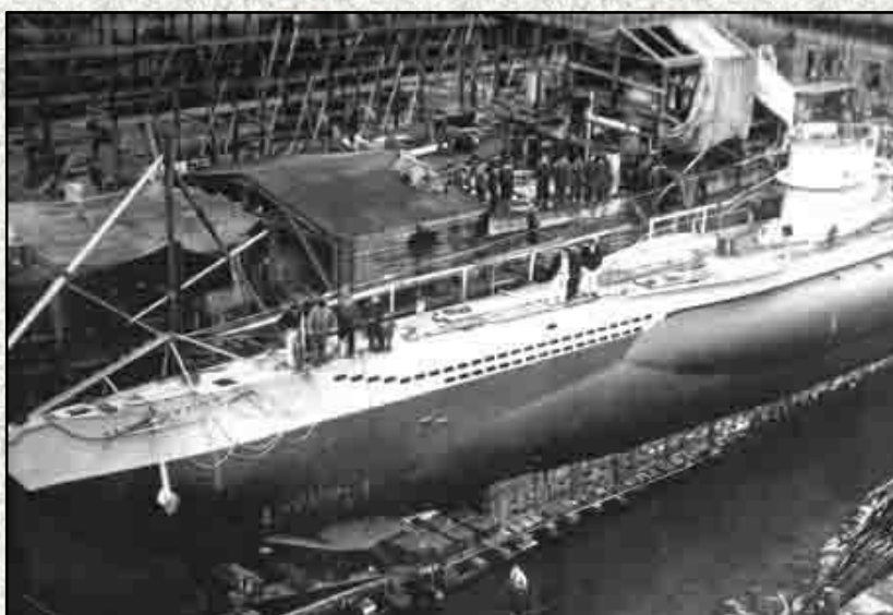
Above (A3): The division between the lighter upper grey and the lower darker grey can clearly be seen on U 69. As was common practice, the whole of U 69's saddle tanks were painted in the lower anti-fouling colour.
