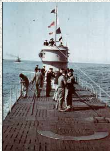
Above (A18): The pristine looking Type IX U 128, with a Hellgrau 50 tower, in May 1941. The freshly-stained wooden deck looks dark, with only a tinge of brown showing through. The metal hatch on the right of the photo, and the C-shaped metal part at the bottom of the photo, have been painted black.
