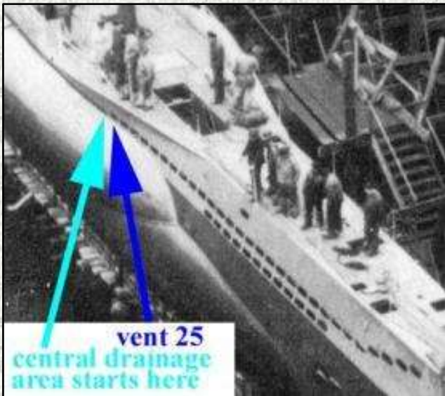
Above (13): Some VIICs such as U 373 above had 25 vents on the top row on the starboard side.
